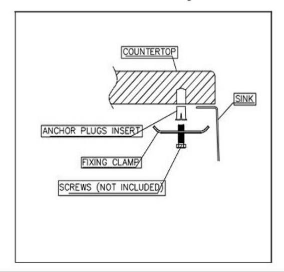
7.Rotate clamp of the clip 90 degrees to the channel and tighten screw clockwise form the center clip using long screw driver.
