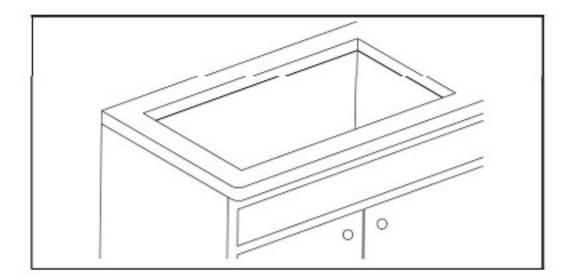
6.Make sure sink rim covers caulking all around and insert screw into the counter top board. Single bowl sink always use 4 clips and double bowl sink use 8 clips.
